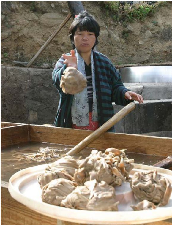
Worker tosses water soaked wood fiber used in hand made paper from soaking tank to transport tray. Thimphu, Bhutan.
