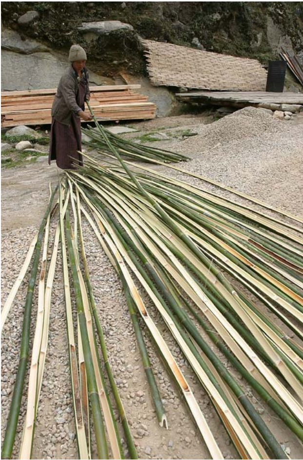
Woman splitting bamboo for weaving panels used for housing. The split bamboo is laid in the road so traffic can flatten it into the pieces used for weaving.
